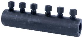
LENTON® LOCK is an in-situ rebar splice from ERICO, requiring no bar-end preparation. It is ideal for new construction, repair or retrofit applications. The Lenton Lock coupler features patented gripping technology that helps provide for the development of full rebar strength and improved overall structural integrity in tension, compression, stress-reversal and dynamic applications.
