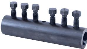
The MBT ET range of couplers provides a cost-effective method of joining reinforcing bars, particularly when the fixed bar is already in place and there is insufficient space for a hydraulic swaging press. This series of couplers is used to connect reinforcing bars of the same size.
